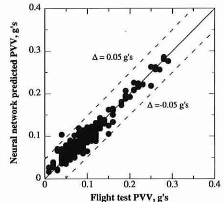
Fig. 18. PVV correlation using hub accelerations along with advance ratio and gross weight.
