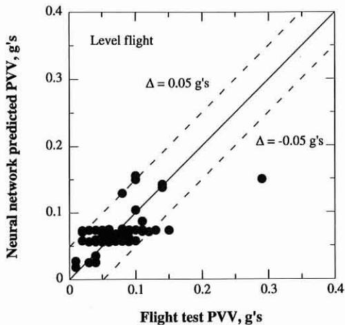
Fig. 5. PVV correlation using advance ratio, level flight.
