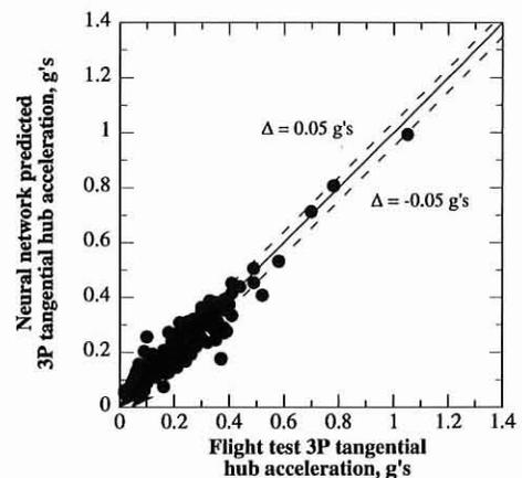
Fig. 13. 3P tangential hub acceleration correlation using maneuver effect factor.
