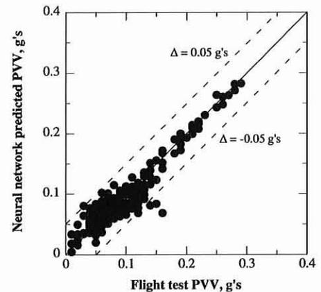
Fig. 17. PVV correlation using hub accelerations and advance ratio.
