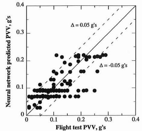
Fig. 16. PVV correlation using hub accelerations.
