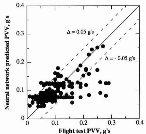
Fig. 8. PVV correlation using advance ratio.
