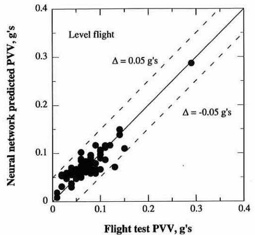
Fig. 7. PVV correlation using advance ratio and gross weight, level flight.
