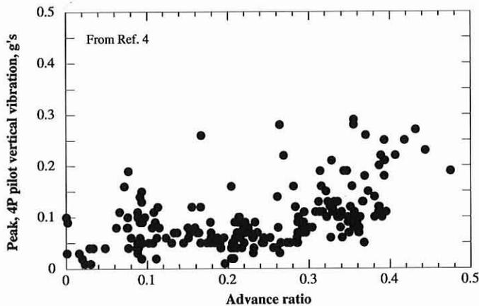
Fig. 4. UH-60A peak, 4P pilot floor vertical vibration, PVV, variation with advance ratio.
