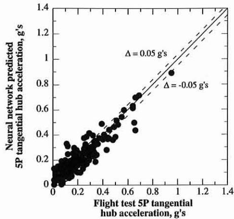
Fig. 14. 5P tangential hub acceleration correlation using maneuver effect factor.
