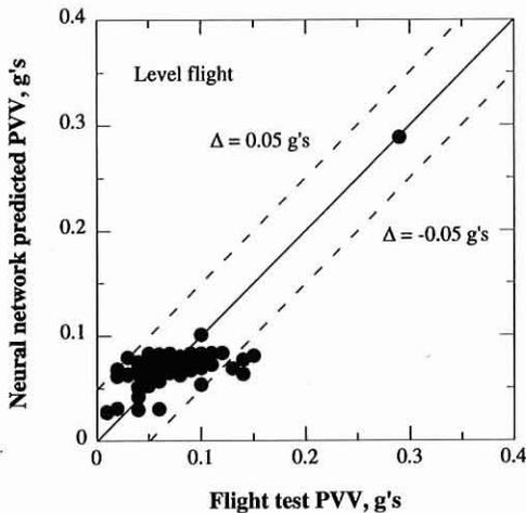
Fig. 6. PVV correlation using gross weight, level flight.
