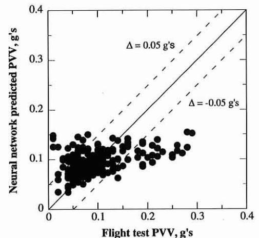
Fig. 9. PVV correlation using gross weight.
