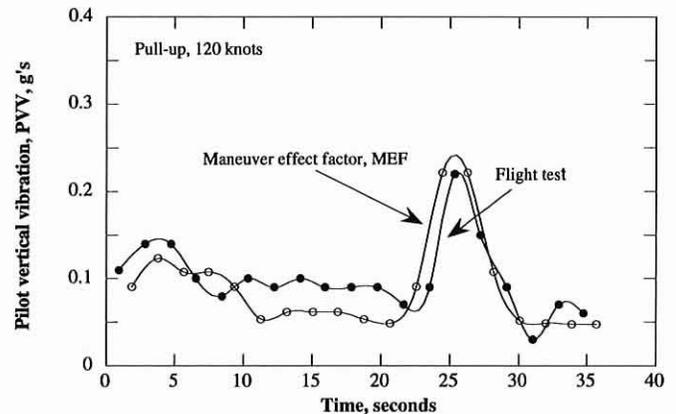
Fig. 12. Quasi-static prediction of PVV using MEF, unsteady pull-up.
