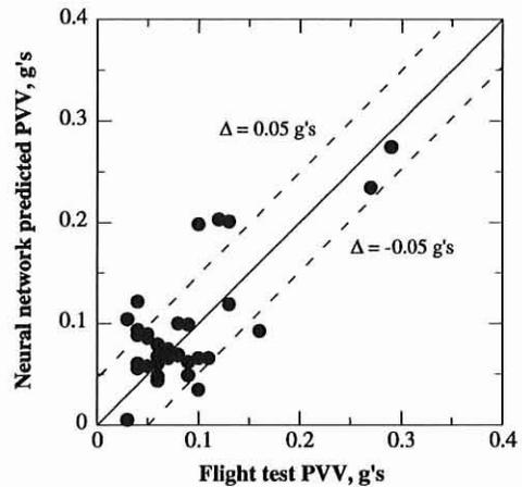
**Fig. 19b. Validation plot, five inputs including hub accelerations, advance ratio and gross weight, associated with Fig. 18.**
